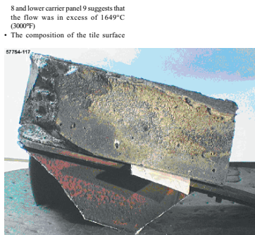
Figure 9.7. Tile Item 57754 bonded to section of carrier panel
