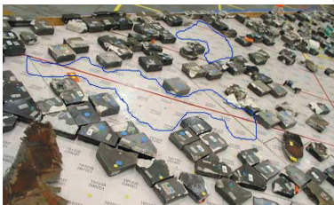
Voids on Left Wing Table
