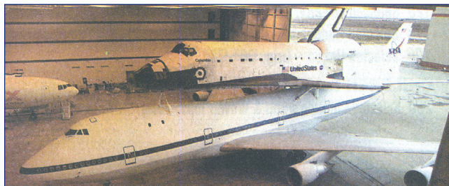
Figure 1.3.4. An Orbiter and SCA partially inside a hangar in Palmdale.
