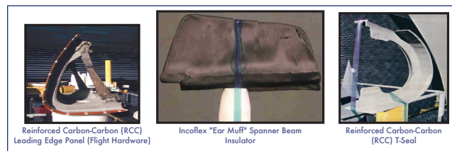
Figure 4-6. Leading edge structural subsystem components matching RCS and ballistics.
